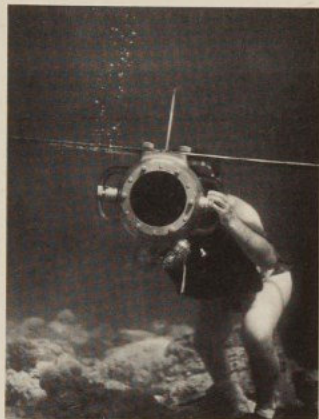
A close-up of our specially designed underwater movie camera. The horizontal wings and the vertical rudder help give it stability.
